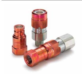
FH Series high pressure, non-spill couplings have flush valves and are designed to minimize spillage and air inclusion when connecting or disconnecting. Couplers and nipples are steel with nitrile seals. Available in 3/8 inch size only, with red finish for easy identification. Will not connect with lower pressure flush face couplings.
